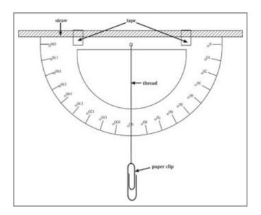
**NOTE**: Some possibilities for Improving: Adding more tick marks for degrees, Adding a handle, Adding a heavier weight such as a large washer, Attaching the Clinometer to the middle of the Compass Rose. Fun to do in spare time in class, when done with an assignment, for **BONUS** points.
